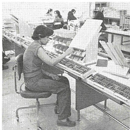
The system starts out with the CPU board being stuffed with chips and parts. Two boards at a time move along the production line.
